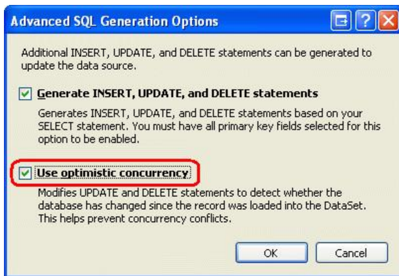
Figure 1: You Can Add Optimistic Concurrency Support from the Advanced SQL Generation Options Dialog Box
