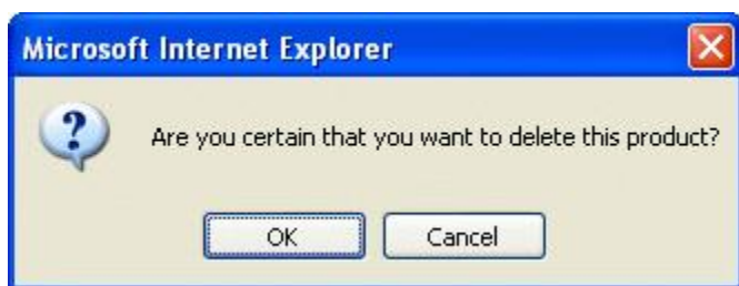
Figure 1: The JavaScript confirm(string) Method Displays a Modal, Client-Side Messagebox
