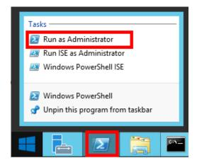
6. Run the **Add-ADSecurityAssessmentTask** command where *<Directory>* is the path to an existing directory used to store the files created while collecting and analyzing the data from the environment.
